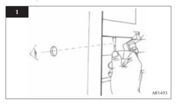
1.2 If there are any extractor fans in adjacent rooms, the test must be repeated with the fans running on maximum and interconnecting doors open.
